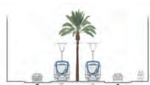
Centrale- couloir tramway arboré
