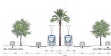
Centrale- couloir tramway arboré
